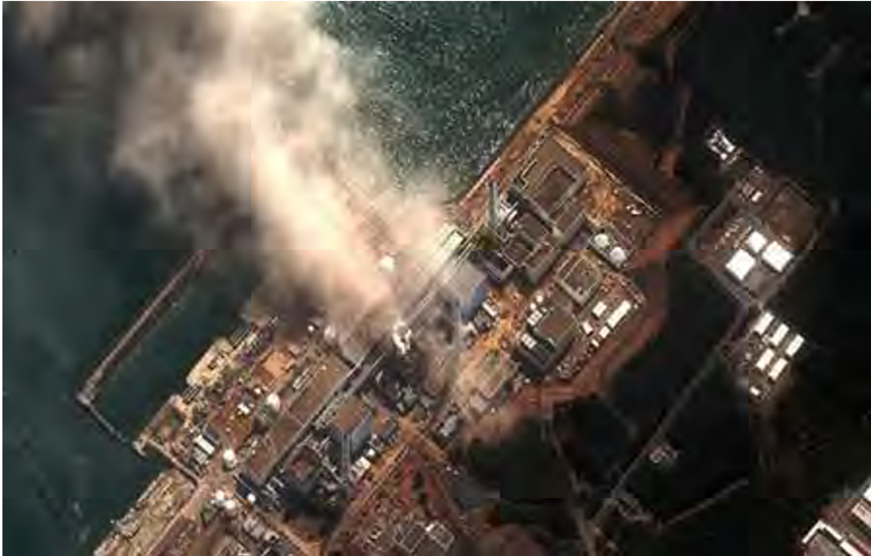
Fig.3 Accident of Fukushima Nuclear Power Plants with Hydrogen Gas Explosion
